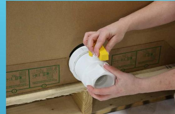
2) Once tight, open the valve as shown. The valve will not cut the membrane so there is no worry about loss of product
