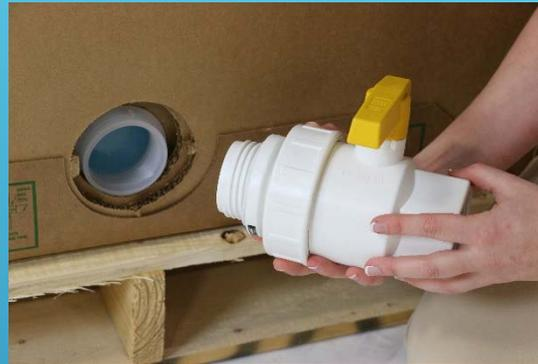
1) Remove bottom cap of the tote and screw the 2" Buttress threads into the evacuation fitment.
