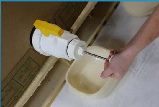
3) Screw the plunger cutter into the backside of the valve. Once tight, push the arrow portion in to puncture the membrane.
